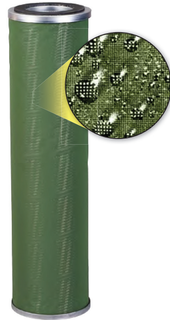
Coalesced water drops from the first stage are shown (above) intruding upon the surface of the PCS Separator Cartridge. The droplets are repelled by the PTFE coated screen, enabling the droplets from passing through. The screen magnification shows how the droplets form on the surface of the PTFE coating.
