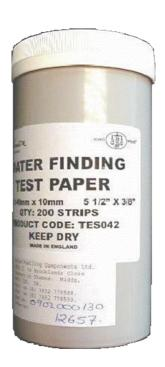
This product is commonly used to detect the presence of larger quantities of free water than would be sought with Shell Water Detector capsules. It is suitable for detecting free water in small tanks and in the bottom of fuel samples. The water finding paper is coated with a brown coating which stays in place when the paper is immersed in fuel, but is removed by any water which may be present, hence exposing the white base underneath.
