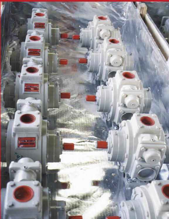
The EBSRAY Model V2000 Rotary Sliding Vane Pump is designed and precision built for efficient handling of LPG, Propane, Butane, DME, Anhydrous Ammonia etc.
