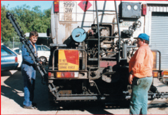
Road Sprayer equipped with EBSRAY G Series Pump & EBSRAY SB Series Spraybar
